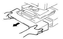
Remove the Projection Lamp from the Lamp Socket.
